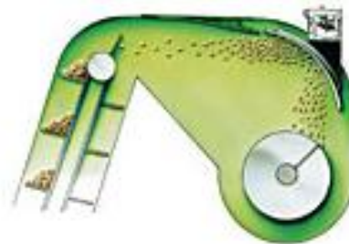
Slika . Senzor masenog protoka na kombajnim John Deere Figure 5. Sensor of weight flow on John Deer combine
