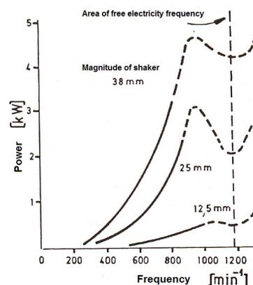
Figure 5. Function diagram of power consumption in correlation with frequency for certain amplitudes
