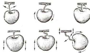
Figure 3. Different fruitage postions during shaking
