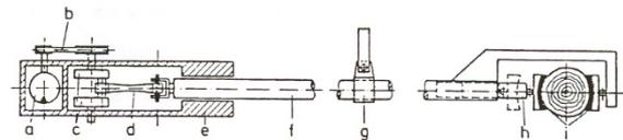
Figure 4. Vibrator with piston and oscillating masses
