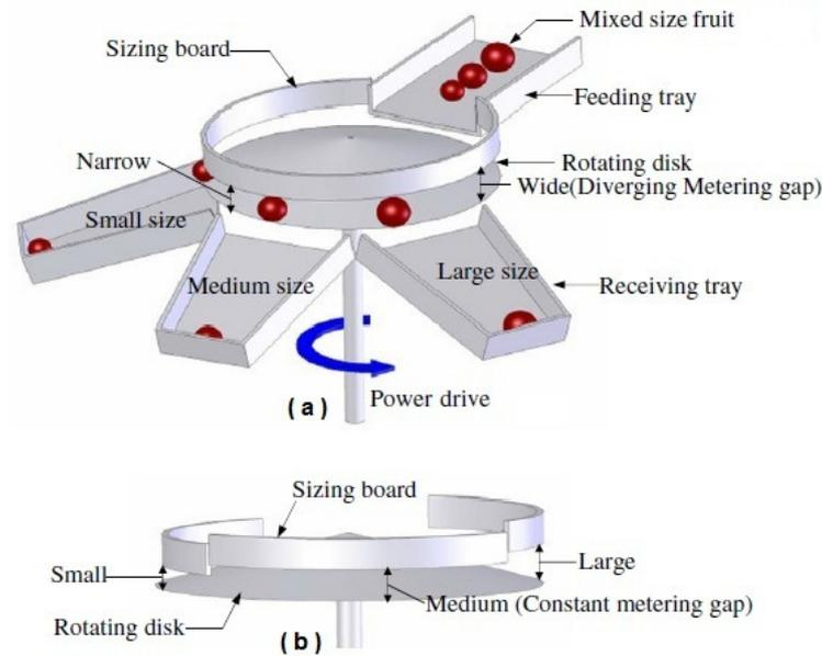
Fig. 1. Model of rotating disc fruit sizing machine. (a) Slope metering gape and (b) step metering gape (Jarimopas et al., 2007).
