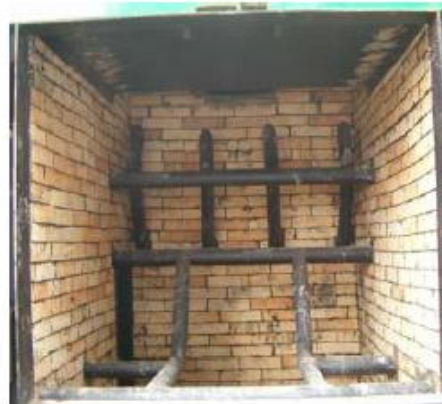
Sl 3 Dvostepena rešetka ložišta kotla termičke snage 300 kW Fig. 3 Twostage grate of firebox boiler with thermic power of 300 kW
